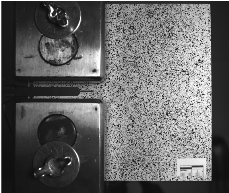
Figure A.23 Unloaded C(T) specimen with 24.5 mm (1.0 in.) in-plane crack
