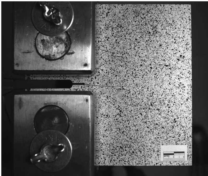
Figure A.62 C(T) specimen with 50.8 mm (2.0 in.) in-plane crack under loading case 3
