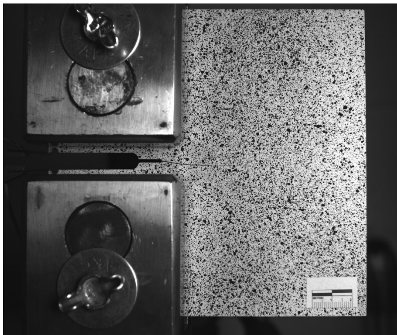
Figure A.52 C(T) specimen with 38.1 mm (1.5 in.) in-plane crack under loading case 5
