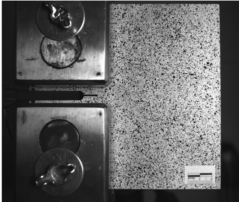
Figure A.14 C(T) specimen with 12.7 mm (0.5 in.) in-plane crack under loading case 3
