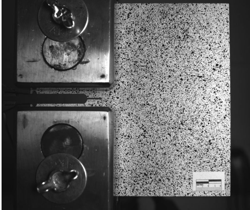
Figure A.24 C(T) specimen with 24.5 mm (1.0 in.) in-plane crack under loading case 1
