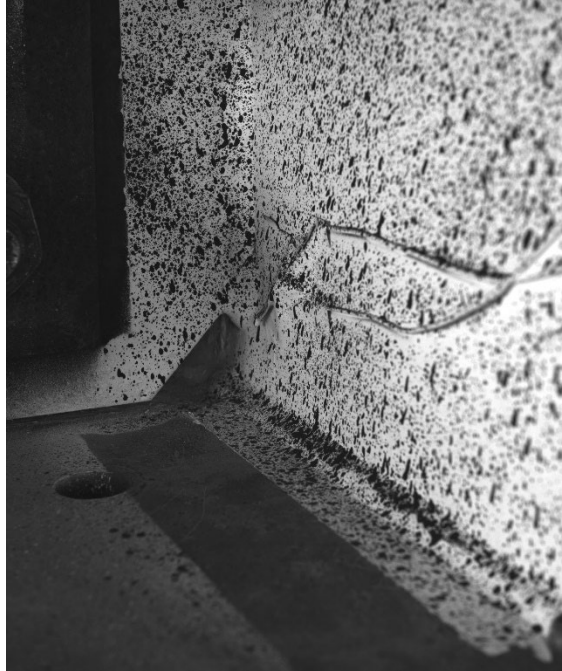
Figure B.14 Out-of-plane specimen under loading case 4
