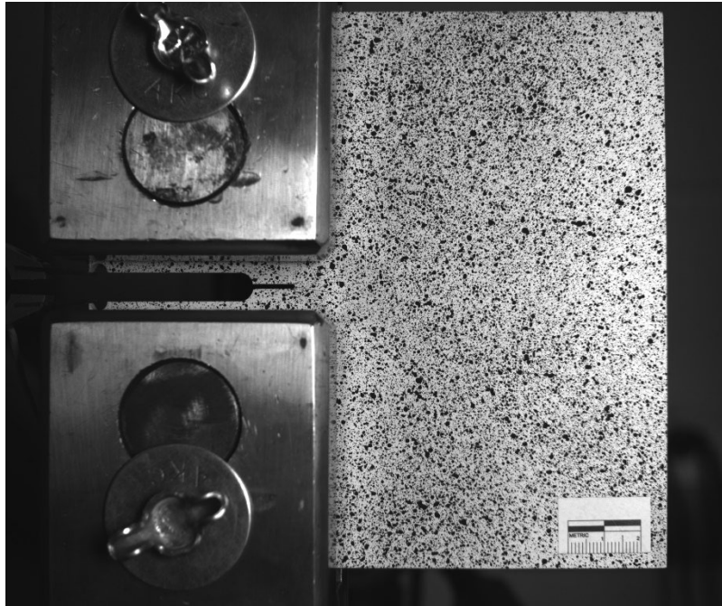
Figure A.27 C(T) specimen with 24.5 mm (1.0 in.) in-plane crack under loading case 2
