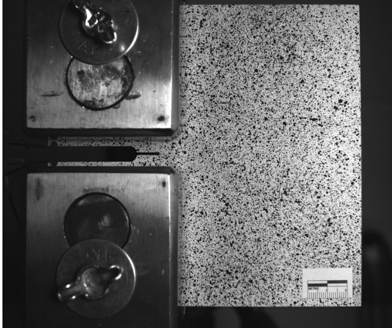
Figure A.39 Unloaded C(T) specimen with 38.1 mm (1.5 in.) in-plane crack
