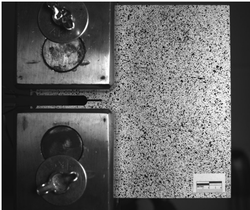
Figure A.46 C(T) specimen with 38.1 mm (1.5 in.) in-plane crack under loading case 3
