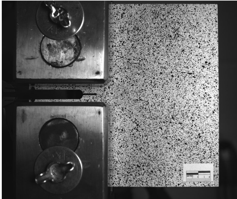
Figure A.33 C(T) specimen with 24.5 mm (1.0 in.) in-plane crack under loading case 4
