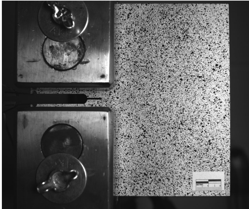
Figure A.43 C(T) specimen with 38.1 mm (1.5 in.) in-plane crack under loading case 2
