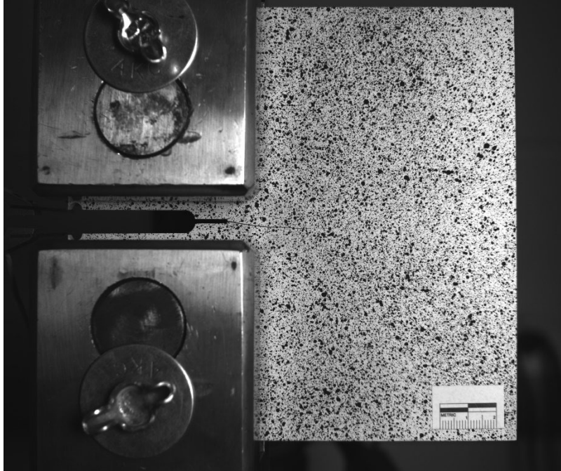
Figure A.49 C(T) specimen with 38.1 mm (1.5 in.) in-plane crack under loading case 4
