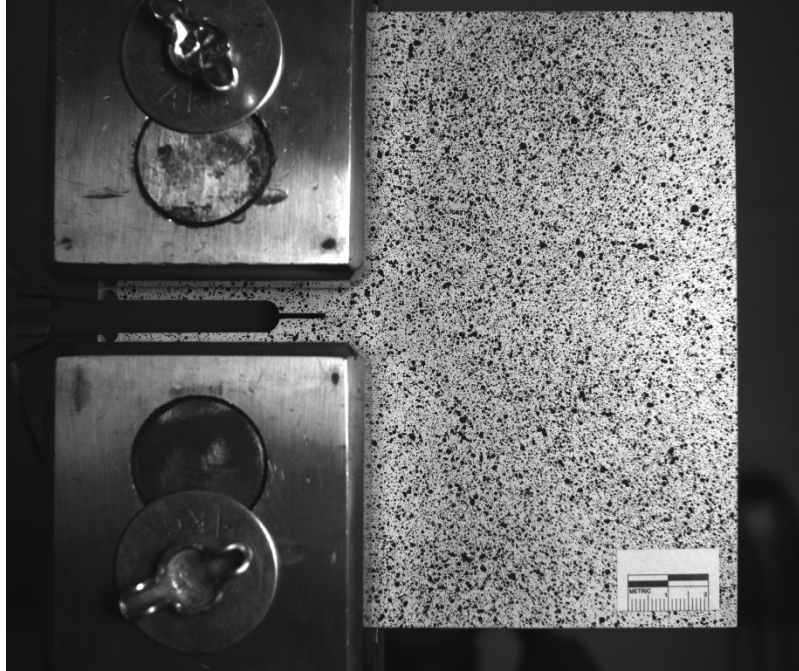
Figure A.20 C(T) specimen with 12.7 mm (0.5 in.) in-plane crack under loading case 5
