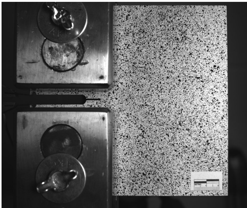
Figure A.17 C(T) specimen with 12.7 mm (0.5 in.) in-plane crack under loading case 4
