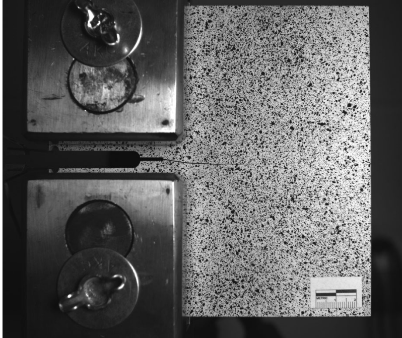
Figure A.59 C(T) specimen with 50.8 mm (2.0 in.) in-plane crack under loading case 2
