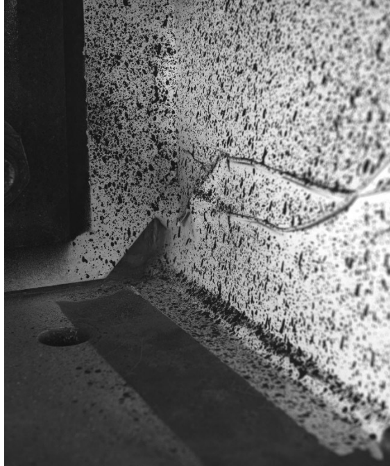
Figure B.1 Unloaded out-of-plane specimen with 44.5 mm (1.75 in.) crack
