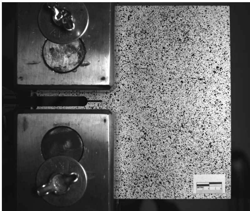
Figure A.30 C(T) specimen with 24.5 mm (1.0 in.) in-plane crack under loading case 3
