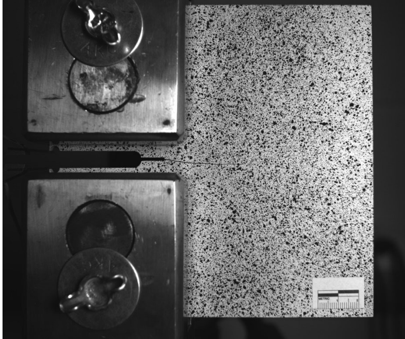
Figure A.55 Unloaded C(T) specimen with 50.8 mm (2.0 in.) in-plane crack
