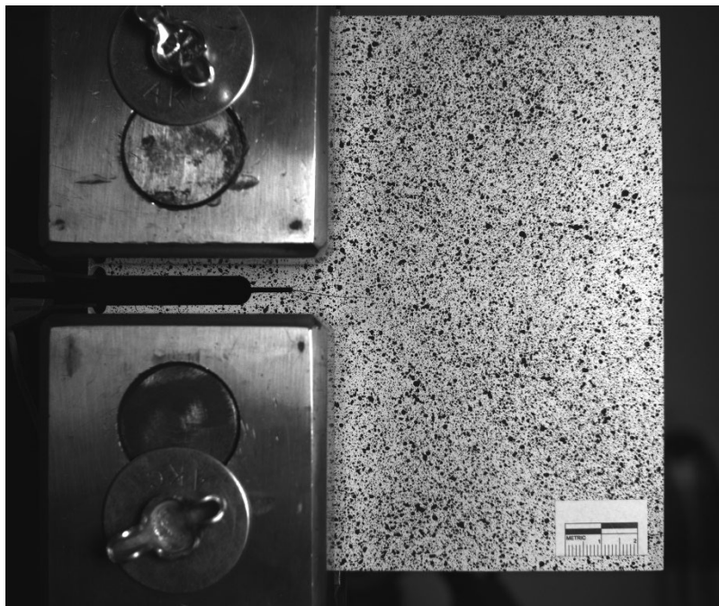
Figure A.36 C(T) specimen with 24.5 mm (1.0 in.) in-plane crack under loading case 5
