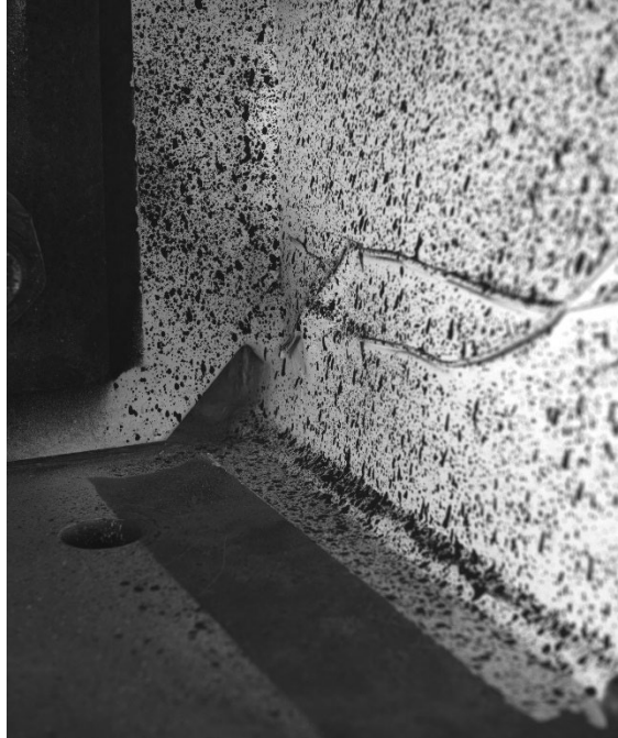
Figure B.18 Out-of-plane specimen under loading case 5
