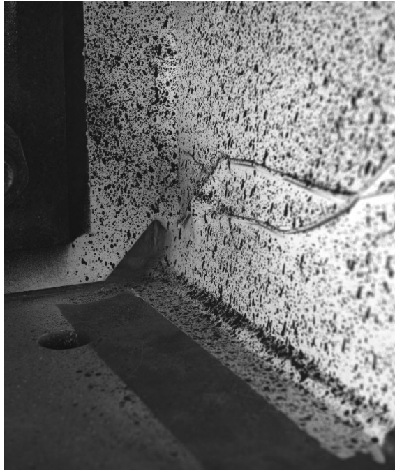
Figure B.22 Out-of-plane specimen under loading case 6
