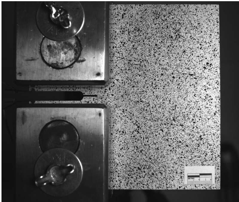
Figure A.40 C(T) specimen with 38.1 mm (1.5 in.) in-plane crack under loading case 1
